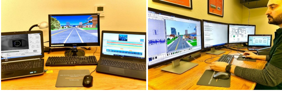
Figure 6.2 Operator workstation for the bicycling simulator. Left: Real-time monitoring of the simulated environment. Right: A researcher designing an experiment in SimCreator.
