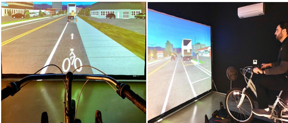
Figure 6.3 Simulated environment in the OSU driving simulator. Left: Participant's perspective. Right: A researcher testing the environment.
